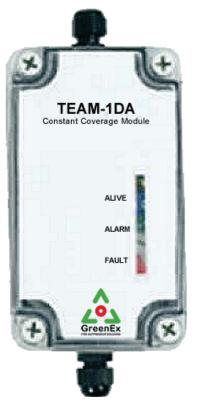
The operation of the Team - 1DA's Rate-of-Rise detector will sense a temperature increase of 40° (f) in less than 60 seconds causing the module to automatically arm and deploy the FST dispensing the aerosol.
