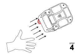
After deploying the GreenPort Portable Fire Suppression Tool (FST) make sure all efforts are maintained to ensure a closed fire room to contain the aerosol. Do Not Ventilate at this point. Allow the FST time to do its job.
